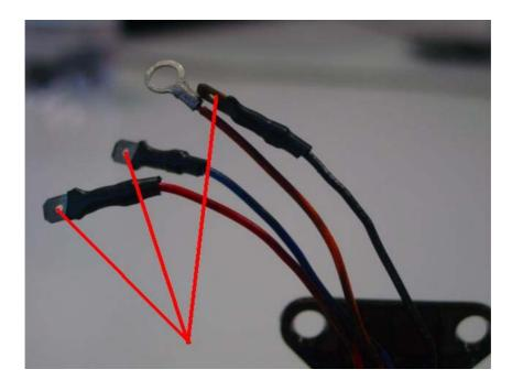
7- Remove the screw at picture and insert the eyelet of the orange wire.
