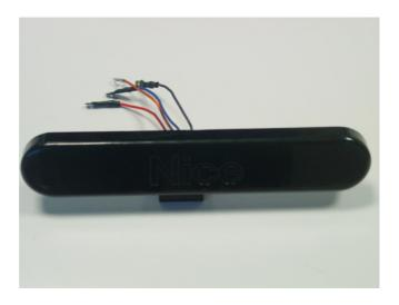
6- Respecting the right colours (black, red and blue), plug the 3 male connectors of the inductive limit switch to the female fastons of the motor.
